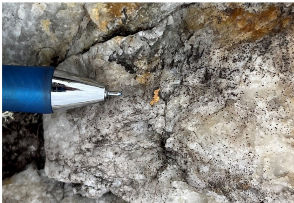
Photo 4 - Rosa Zone. Sub-horizontal extensional quartz vein with visible gold. Grab sample returning 19.75 g/t Au (sample F689432).
