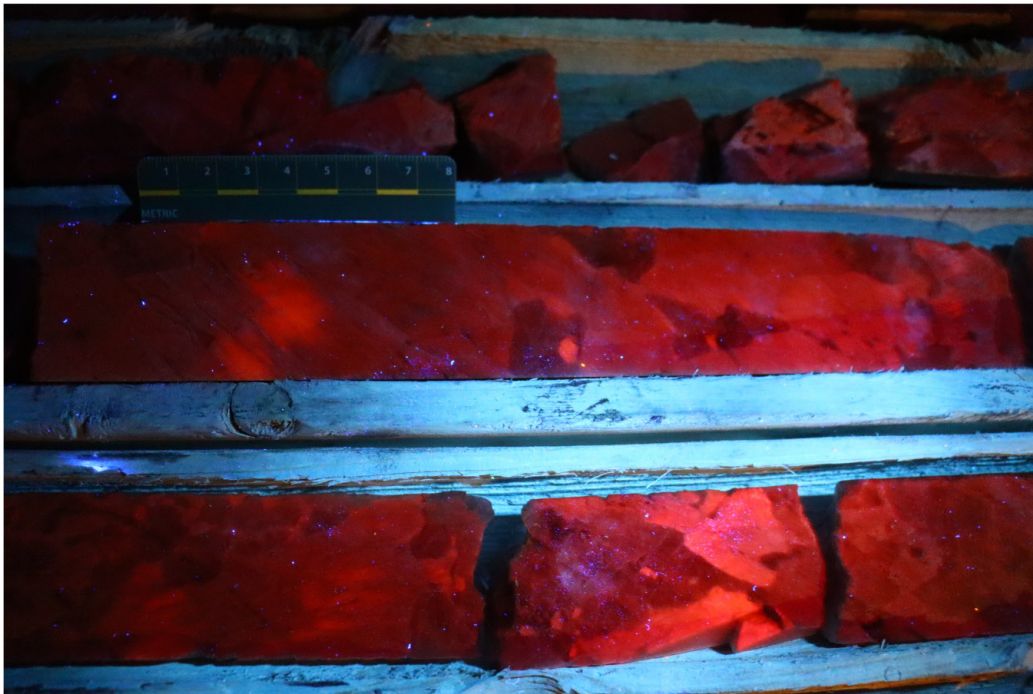
Photo 3: Very coarse white spodumene crystals in Hole GAL24-020 (this picture: from 126.5 m to 127.7m). UV light. Spodumene crystals appear in red.
