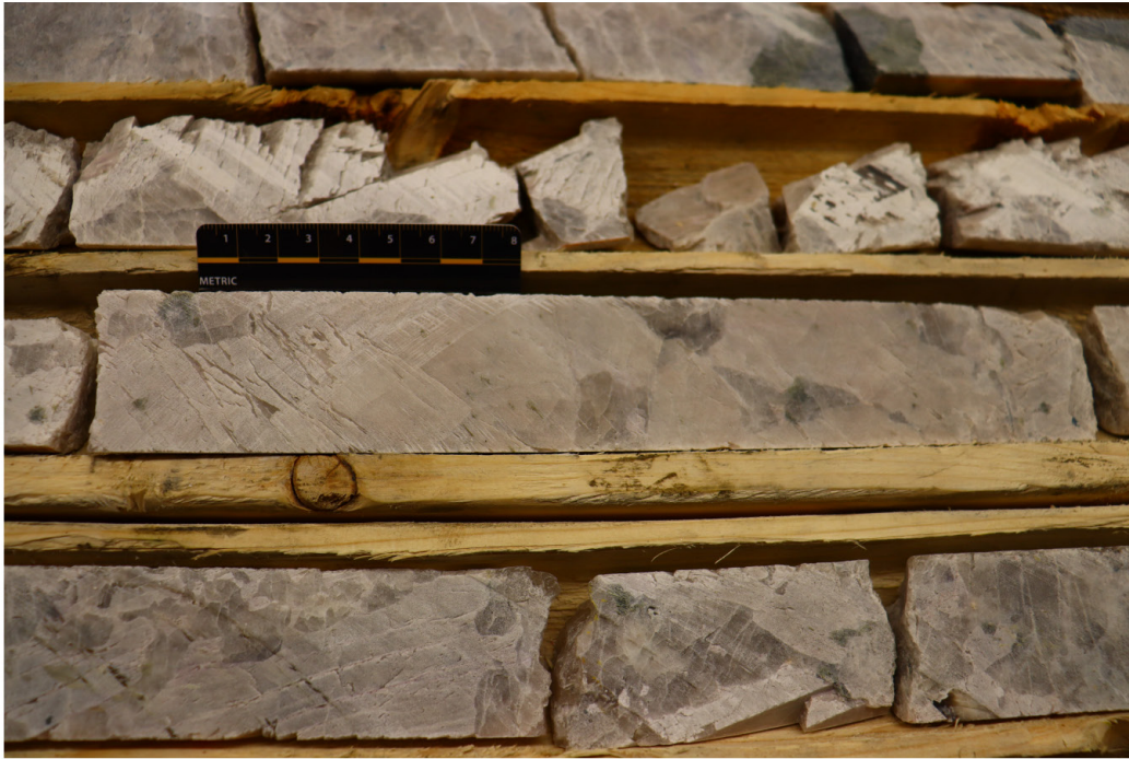
Photo 2: Very coarse white spodumene crystals in Hole GAL24-020 (this picture: from 126.5 m to 127.7m). Natural light.
