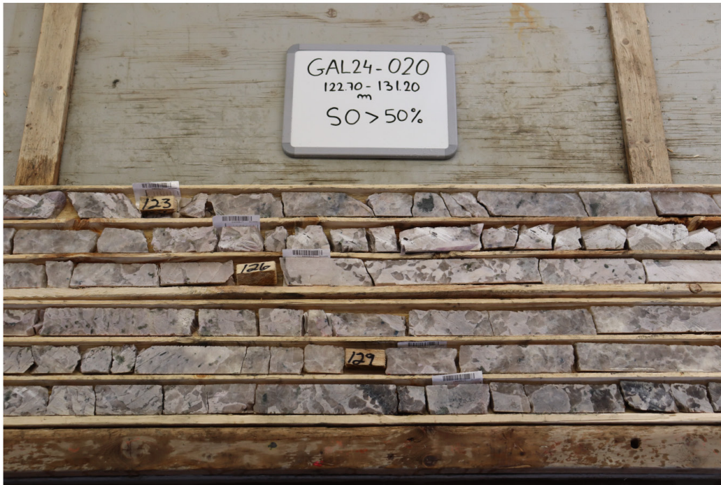
Photo 1: Spodumene pegmatite interval over 71.85 metres (from 75.85 m to 147.7 m) in Hole GAL23-020 with >50% of very coarse white spodumene crystals (this picture: from 122.7 m to 131.2 m).
