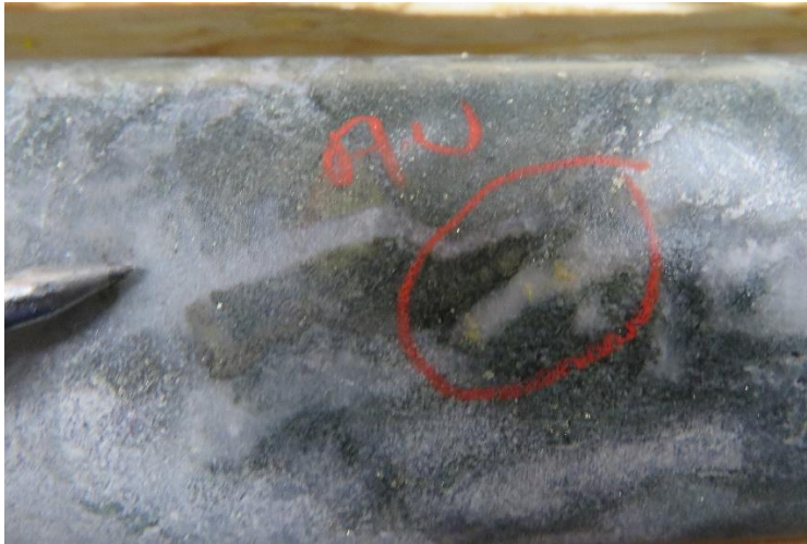
Hole ELM19-001: Native gold in quartz vein at 87.15 m. Sample Y104333: 18.4 g/t Au over 0.80 m
