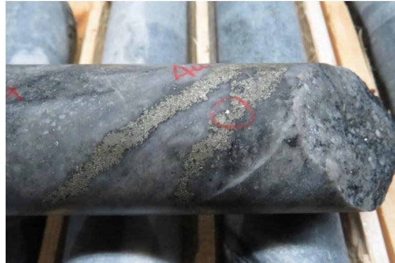
Hole ELM19-006: Native gold grain in a pyritic stringer in felsic intrusion at 70.7 m. Sample Y103973: 121.0 g/t Au over 0.50 m
