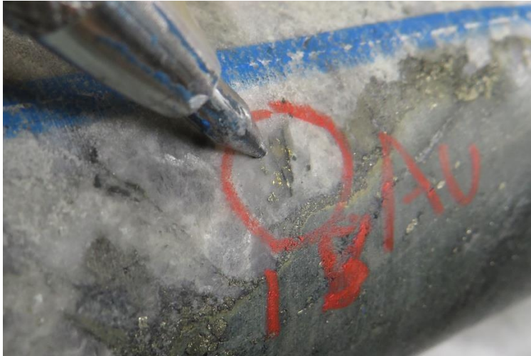
Hole ELM19-005: Native gold in a quartz vein at 28.47 m with up to 20% pyrite. Sample Y103830: 29.8 g/t Au over 0.50 m
