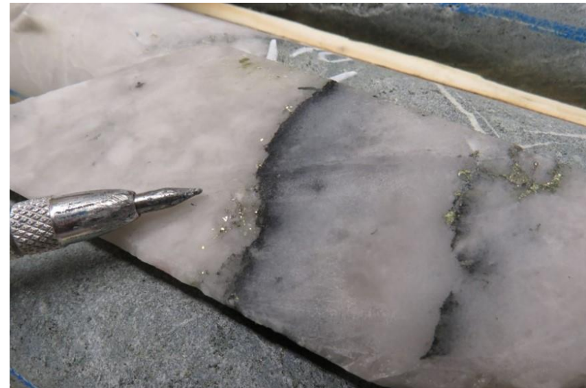
Hole ELM19-004: Native gold in milky quartz vein with tourmaline selvages at 16.2 m. Sample Y103725 : 28.7 g/t Au over 0.50 m
