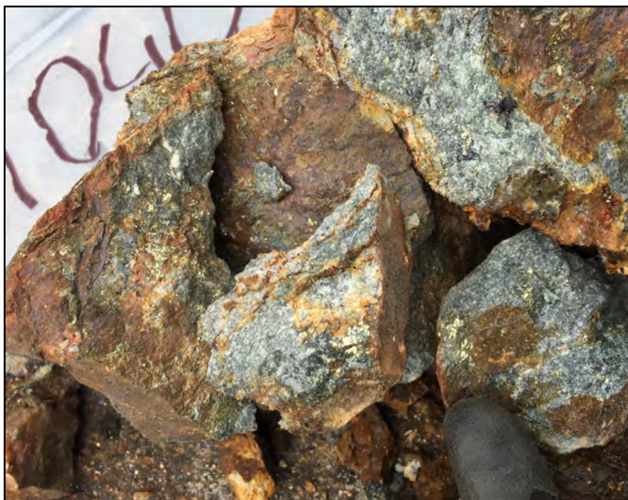
Photo 2: Maschakw Au-Ag-Cu Prospect, hematized sericitized paragneiss with chalcopyrite, 3.02 g/t Au, 35.3 g/t Ag, 1.29% Cu (grab sample Y104081)
